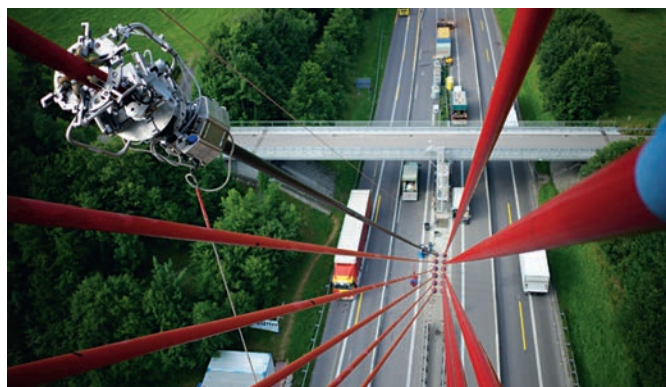
Fig. 9. Wrapping robot on painted cables
