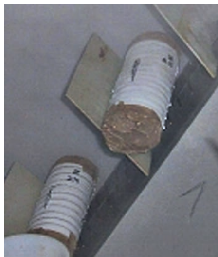
Fig. 4. Samples in the salty fog test
