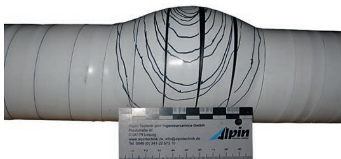
Fig. 8. Test sample subjected to 30 bar interior pressure under the wrapping
